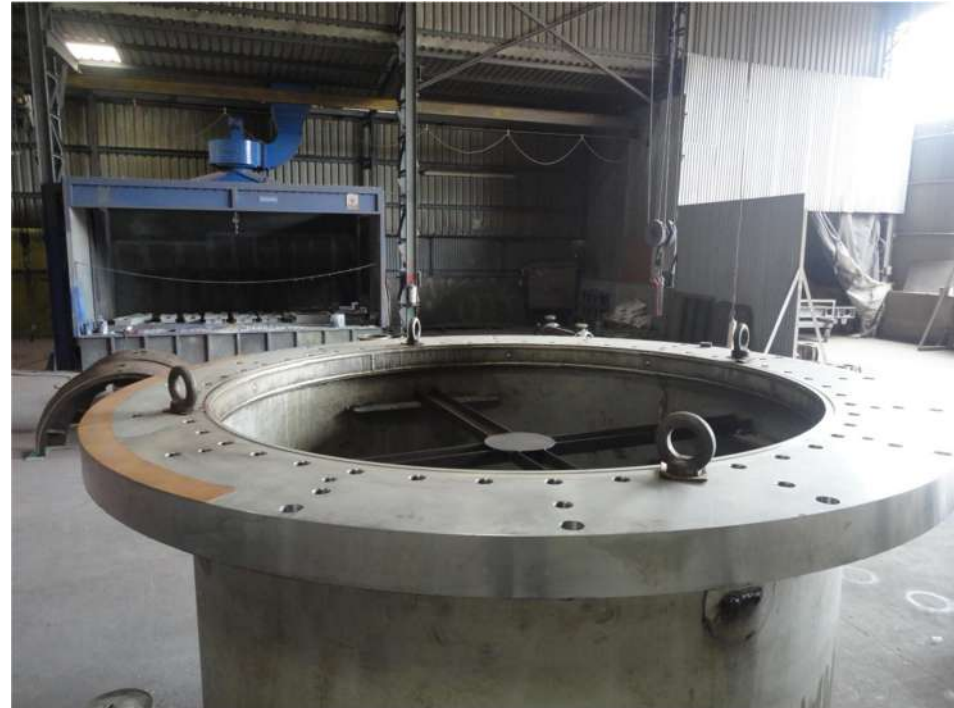
CONDENSATE PUMP BARREL
