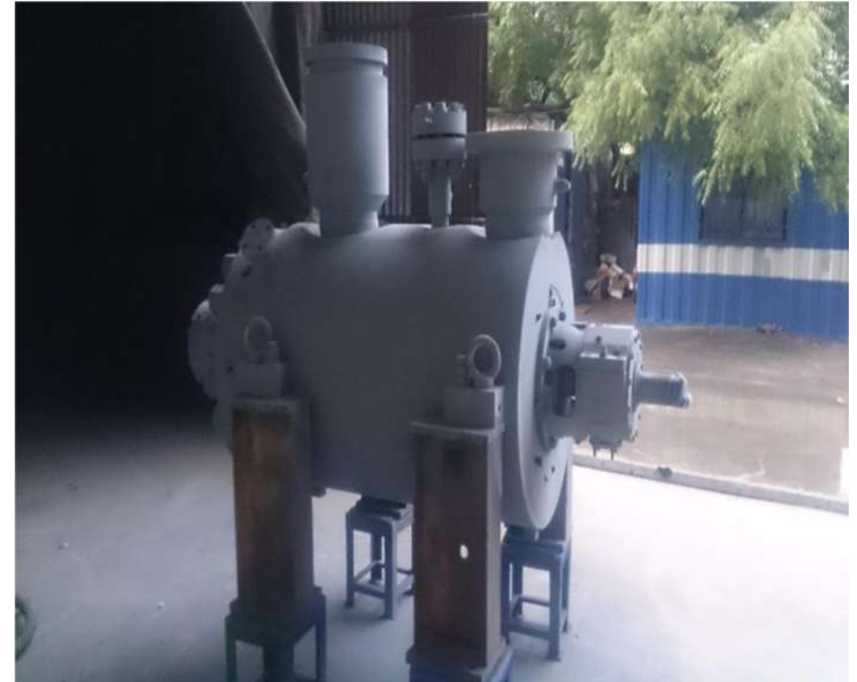
HIGH PRESSURE BOILER FEED PUMP
