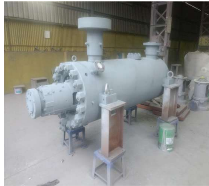
HIGH PRESSURE BOILER FEED PUMP
