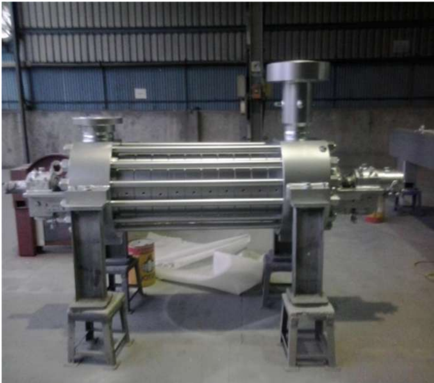
HIGH PRESSURE BOILER FEED PUMP
