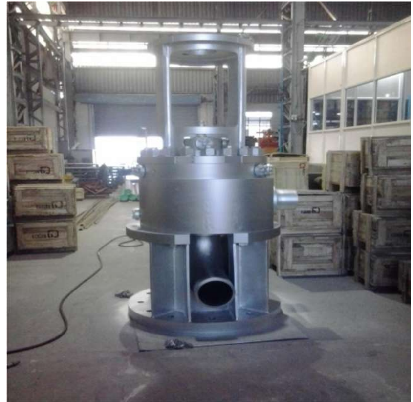
NUCLEAR SHUTDOWN COOLING PUMP
