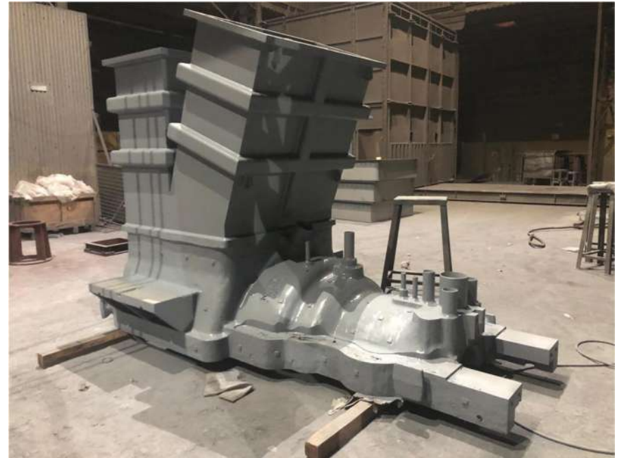
STEAM TURBINE CASING
